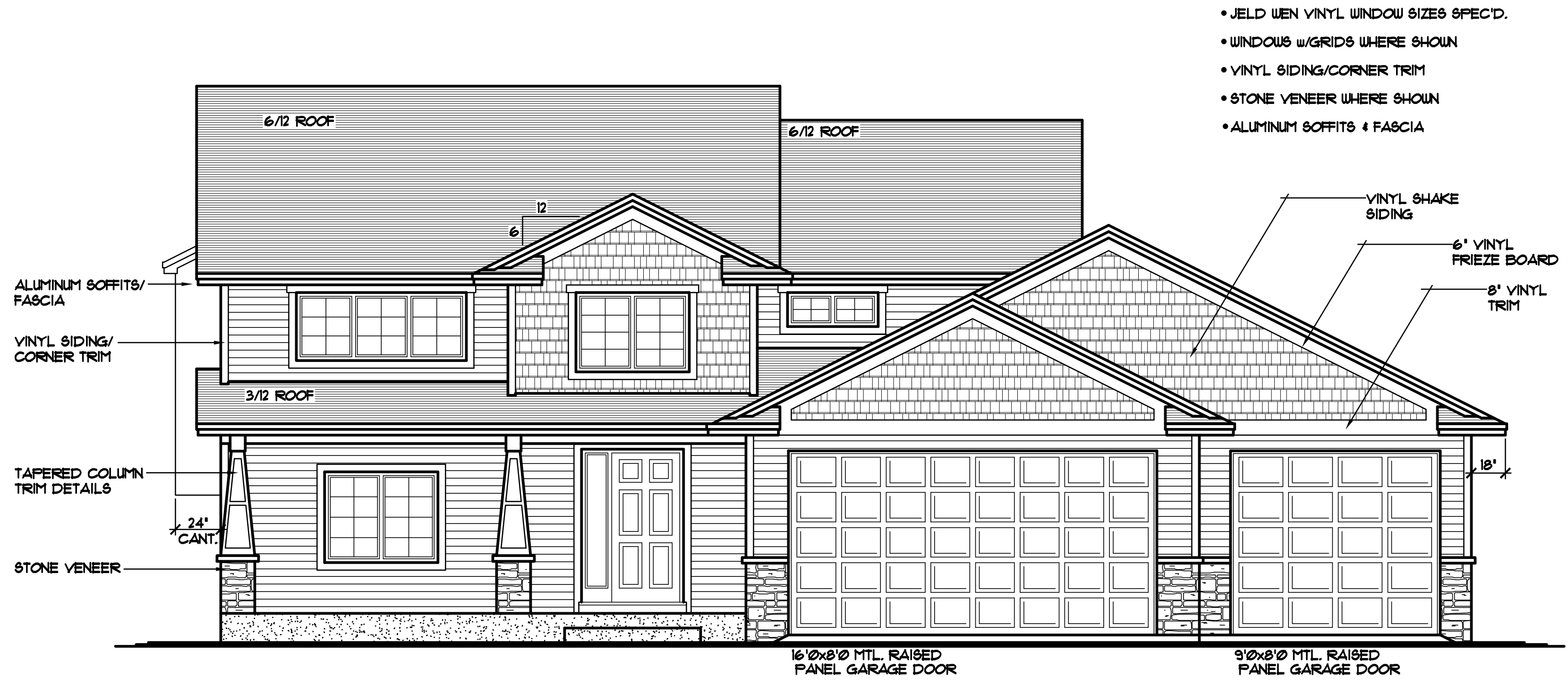
FRONT ELEVATION 1/4"=1'-0" 1029 SQFT. MAIN LEVEL
